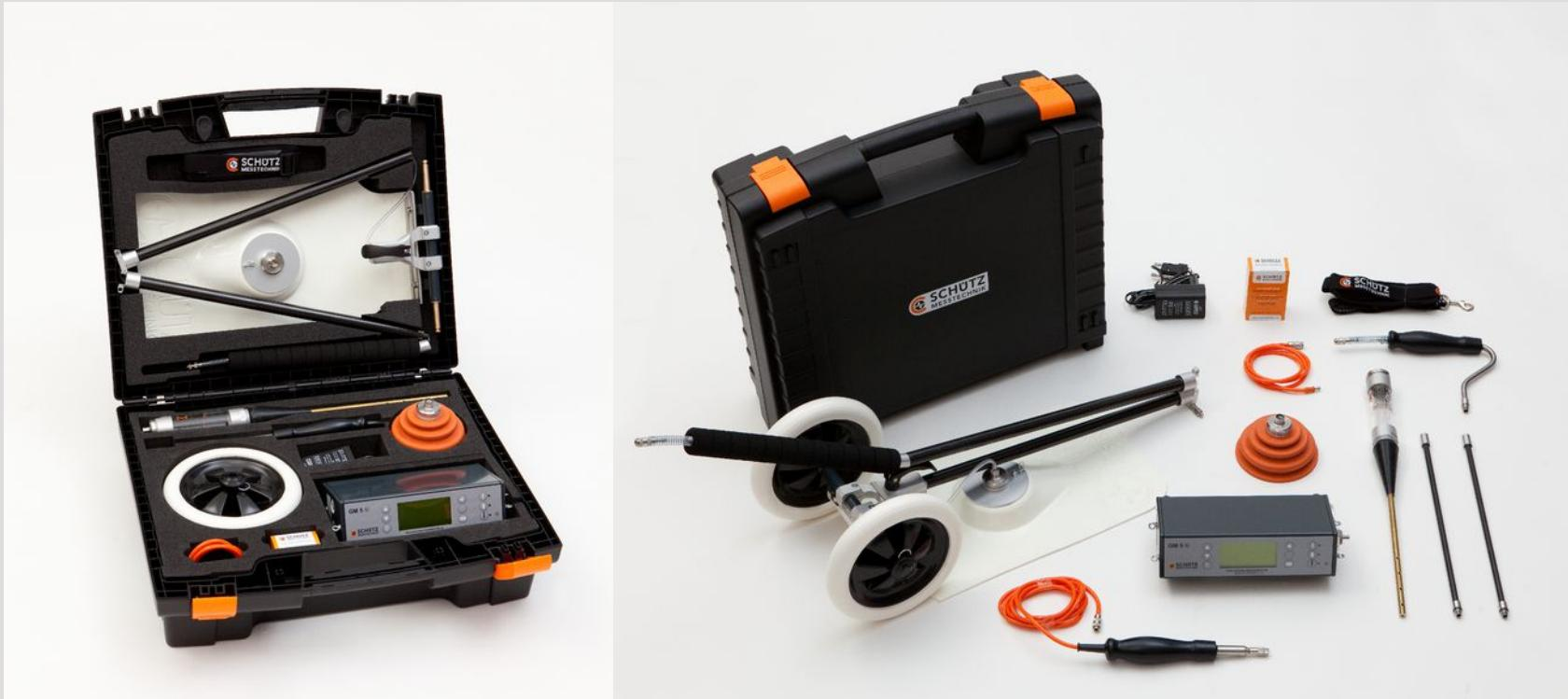
**Case-copmplete set with bell and borehole probe with screwable tube and foldable carpet probe. All probes are weight-optimized and made of carbon fiber.**
